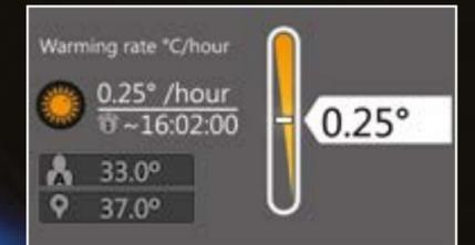
**Custom Warming** is adjustable within a hundredth of a degree from  $0.05^{\circ} \text{C}$  to  $0.5^{\circ} \text{C}$  per hour. Altrix will calculate estimated time for each warming rate option.
