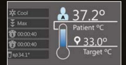
**Therapy Screen** provides key treatment data throughout temperature management, including patient temperature, target temperature, water temperature, and timing.
