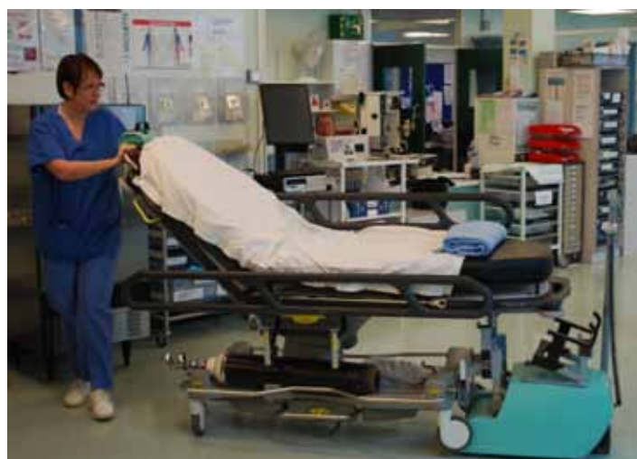
Figure 5 External device using a remote control option – far superior to manually pushing but still a long wheelbase and distance to the drive wheel
