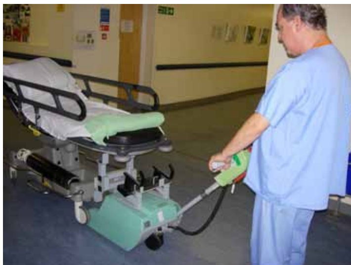
Figure 4 External driving device – two trolley wheels raised off the floor. How does the operator calculate how much weight is being applied to the machine?
