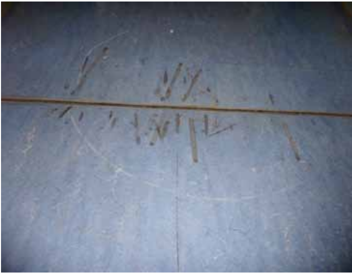
Figure 1 Scuff marks - Start of the Incline – loss of traction
